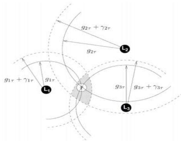
Fig. 1: Multilateration with geographic distance constraints. [7]
