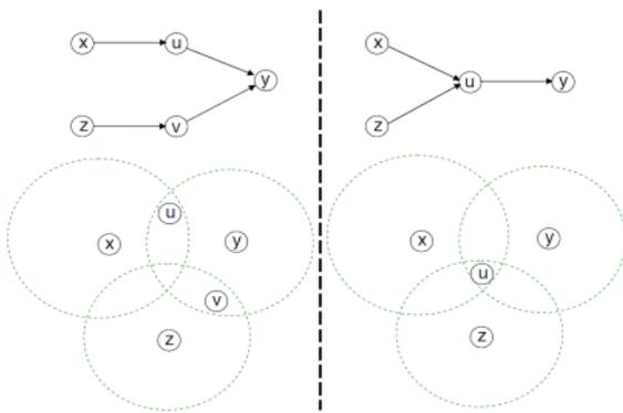
Fig. 3: Router aliases: Accuracy improves from (a) to (b) as v is identified as an alias for u. [8]
