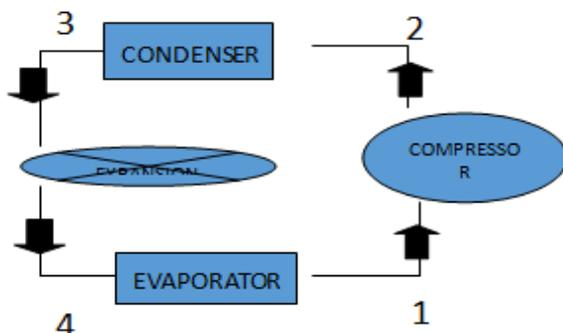
Fig. 5: Vapour Compression Cycle
