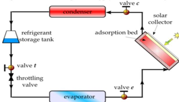
Fig. 4: Schematic diagram of the solar adsorption cooling system by SnehaPatil et al (2015)
