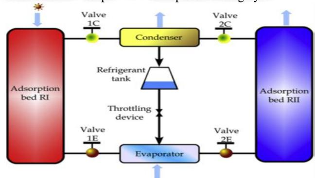
Fig. 3: Diagram of the constant temperature adsorption cooling cycle by Hassan et al (2012)
