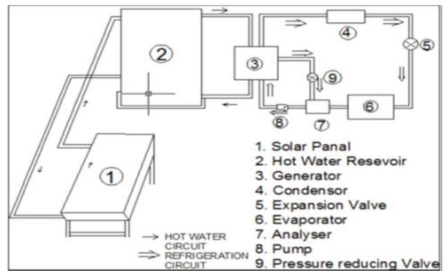
Fig. 2: Experimental set-up of Solar Cooling System by SrinivasaRao et al (2013)
