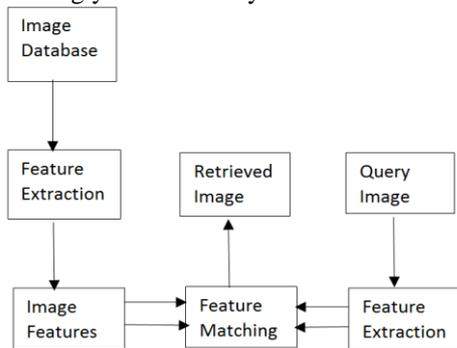
Fig. 1: Block diagram of CBIR system
