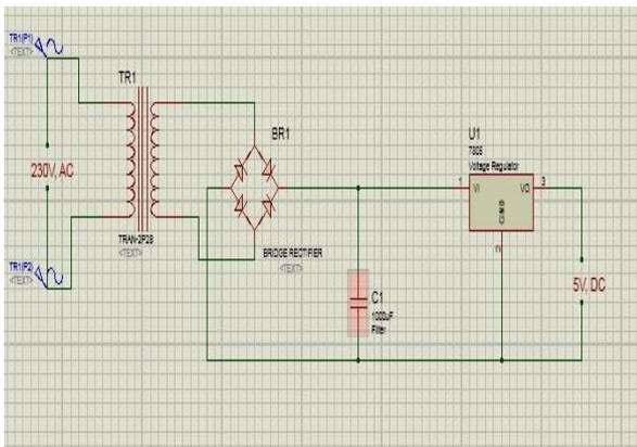
Fig. 1: Components of a typical linear power supply
