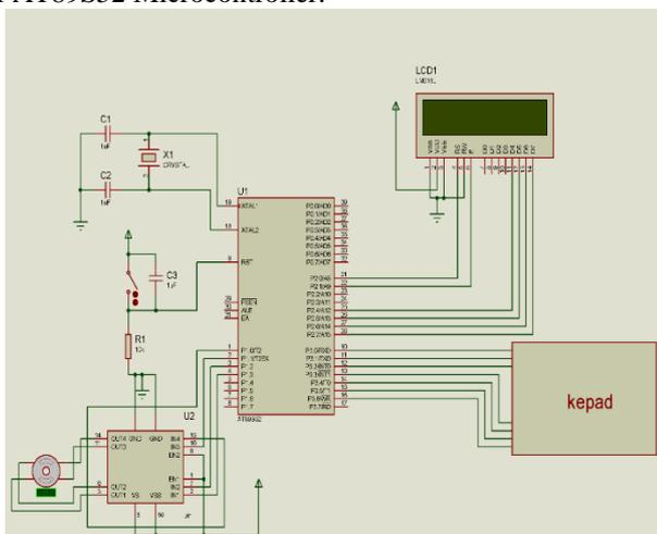
Fig. 2: Circuit of PC- based stepper motor controller
