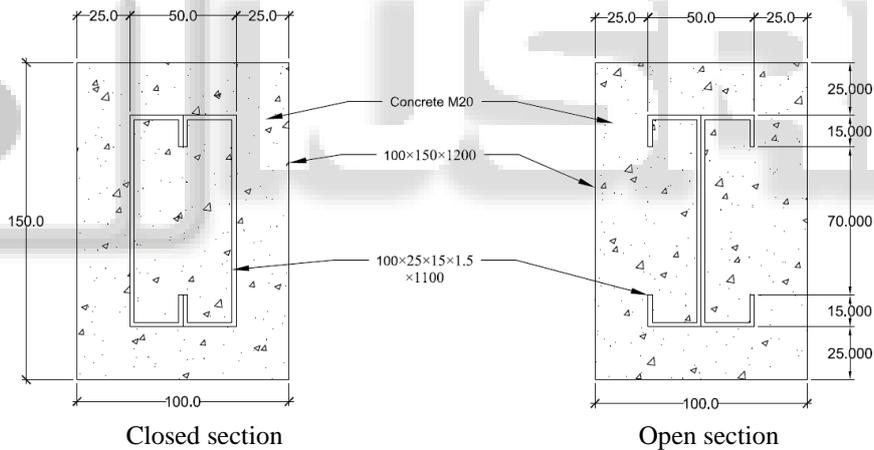
Fig. 3.1: Typical cross sectional details of beam specimens (all dimensions are in mm)
