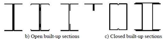
Fig. 1.1: Various types of Cold-Formed Sections
