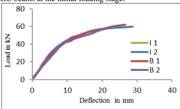
Fig. 4.1: Load-Deflection response of encased beams
