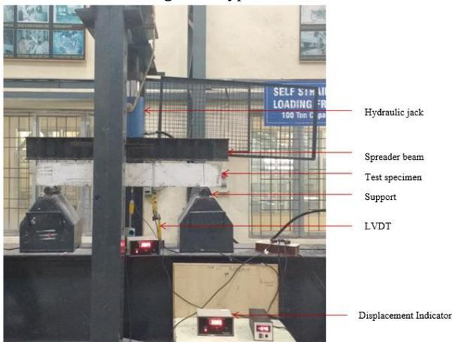
Fig. 3.2: Two-point loading test setup
