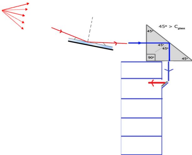
Fig. 3: Orientation and inclination of mirrors and prisms and the path followed by sunlight
