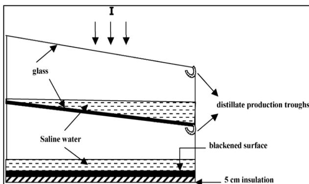
Fig. 5: Schematic Diagram of Simple Double Basin [10]
