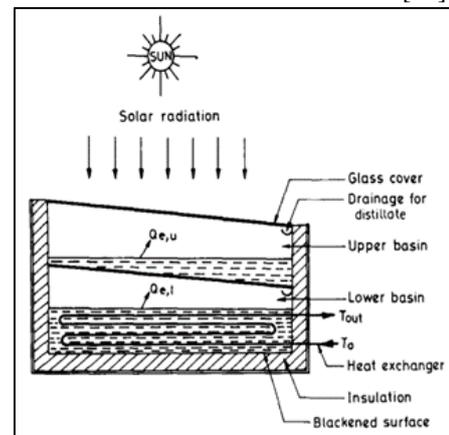
Fig. 10: Schematic Diagram of Double Basin Solar Still with Heat Exchanger [18]
