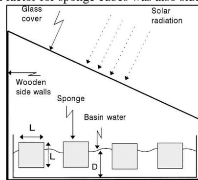
Fig. 2: Schematic Diagram of Solar Still with Sponge Cubes [5]
