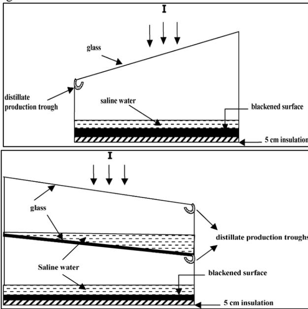
Fig. 7: Schematic Diagram of Simple Single Basin and Double Basin Solar Still with Same Basin Area [14]
