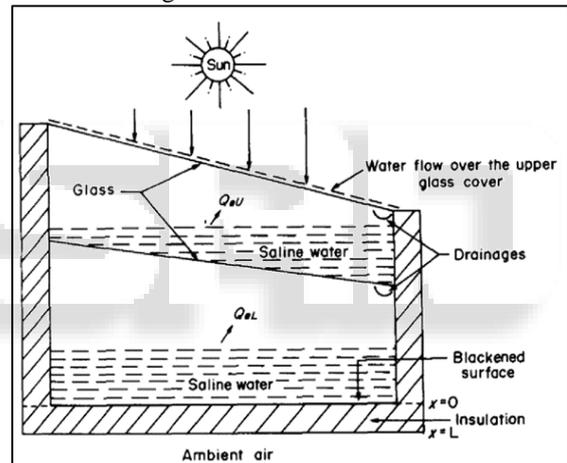
Fig. 9: Experimental view of Water Flowing over Glass Cover of Double Basin Solar Still. [16]
