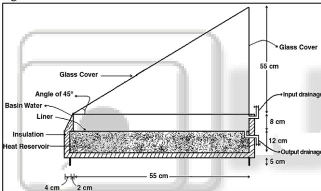
Fig. 4: Schematic Diagram of Solar Still with Sandy as Heat Reservoir [8]
