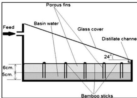
Fig. 3: Schematic Diagram of Solar Still Used with Porous Fins in Basin [7]
