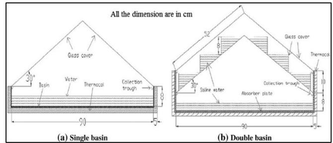
Fig. 8: Experimental view of (a) Double Slope Single Basin Solar Still and (b) Double Slope Double Basin Solar Still. [15]
