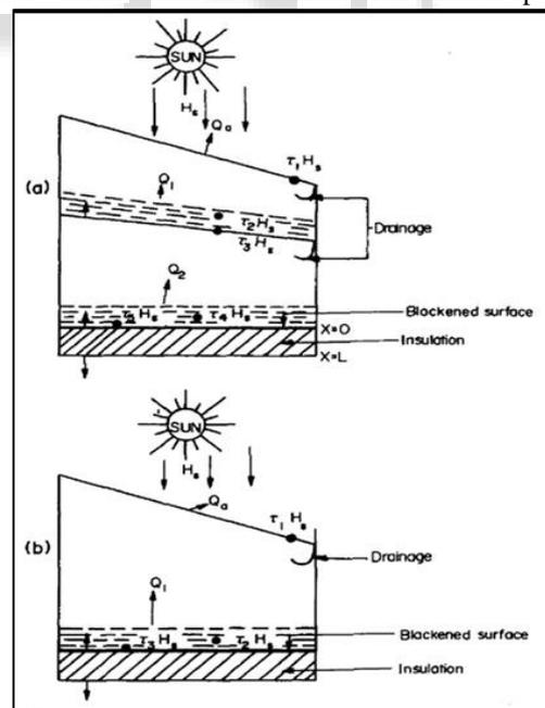
Fig. 6: Experimental view of (a) Single Basin Solar Still and (b) Double Basin Solar Still [13]
