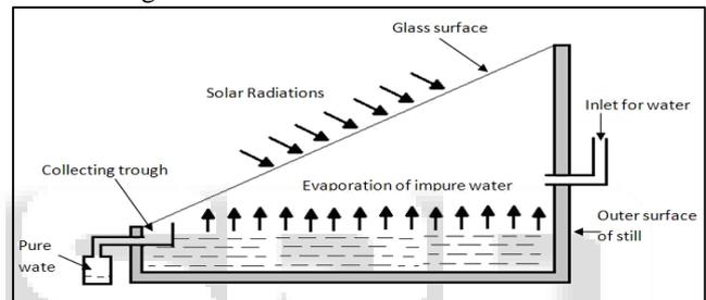
Fig. 1: Schematic Diagram of Conventional Solar Still [4]
