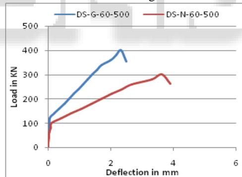
Fig. 7: Load vs Deflection curves for 60mm dia DSTC and 500 mm length
