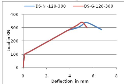
Fig. 10: Load vs Deflection curves for 120mm dia DSTC and 300 mm length
