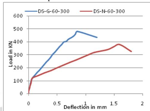
Fig. 6: Load vs Deflection curves for 60mm dia DSTC and 300 mm length
