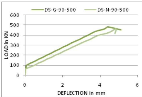
Fig. 9: Load vs Deflection curves for 90mm dia DSTC and 500 mm length
