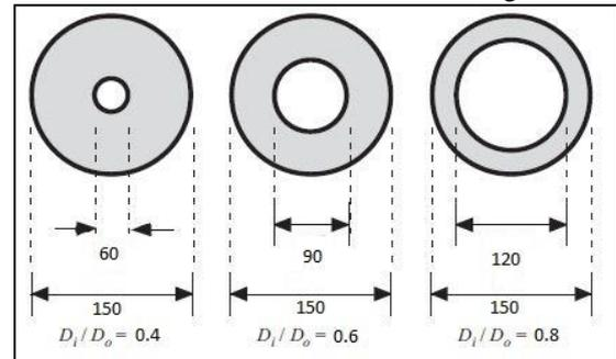
Fig. 3: Cross-section of the specimen
