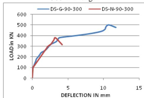
Fig. 8: Load vs Deflection curves for 90mm dia DSTC and 300 mm length
