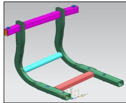
Fig. 2: Isometric view of the mounting bracket
