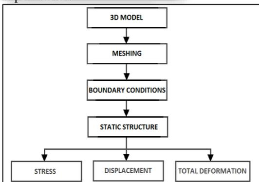
Fig. 4: Flow chart for Static Structural analysis
