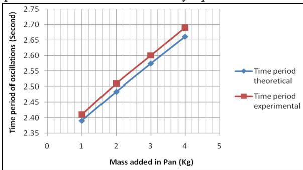
Fig. 6: Comparison of Theoretical and Experimental Time Period for L<sub>1</sub> = 44.5 cm
