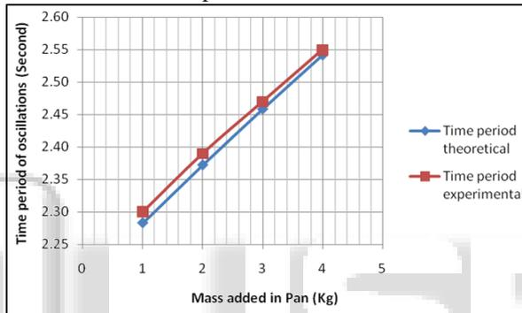
Fig. 5: Comparison of Theoretical and Experimental Time Period for L<sub>1</sub> = 42.5 cm
