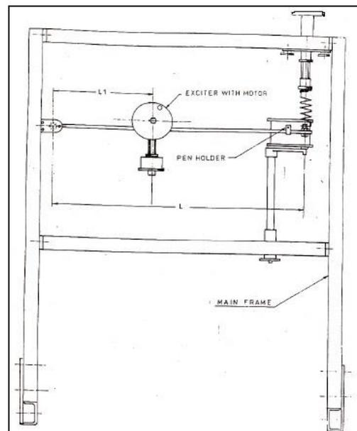
Fig. 1: Experimental set up for time period measurement
