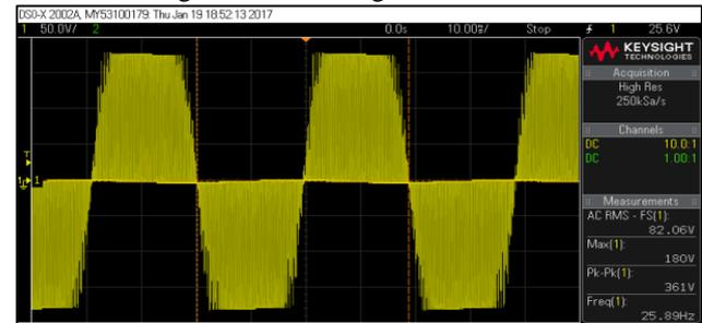
Fig. 6: Phase voltage at 700 RPM
