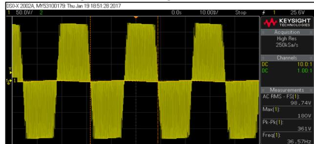
Fig. 5: Phase voltage at 1020 RPM
