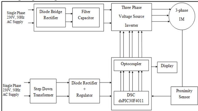
Fig. 1: Block diagram of three phase induction motor using Digital signal controller.
