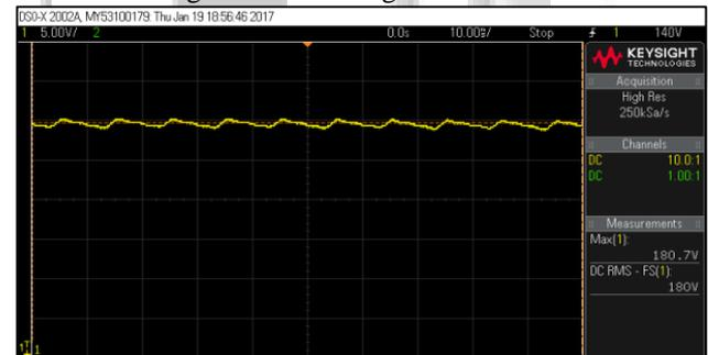
Fig. 7: DC link voltage with ripple
