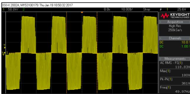
Fig. 4: Phase voltage at 1380 RPM
