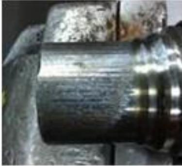
Fig. 4: Universal Joint Spalling
