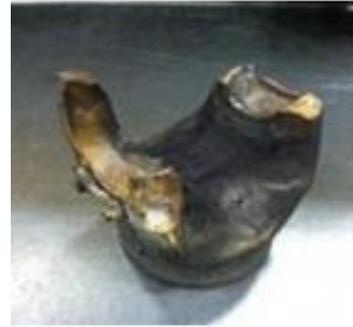
Fig. 7: Weld Yoke Failure <sup>(5)</sup>
