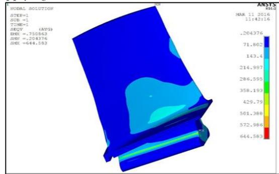
Fig. 5: Von – mises stress with RPM - 16000
