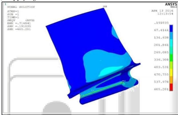
Fig. 7: Von-mises stress with RPM – 15500
