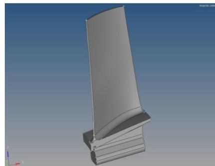
Fig. 2: Compressor Blade Modelled in Uni-graphics
