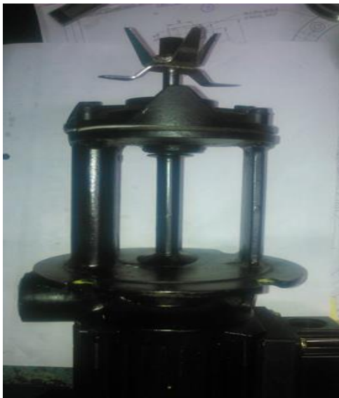
Fig. 6: Assembly of crusher with Vertical Submerged Pump
