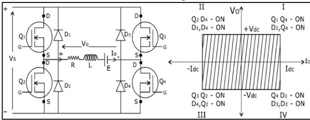
Fig. 3: Circuit diagram of H-Bridge MOSFET Chopper
