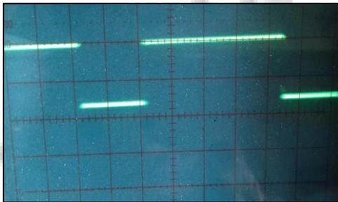
Fig. 5: H-Bridge gate drive pulses
