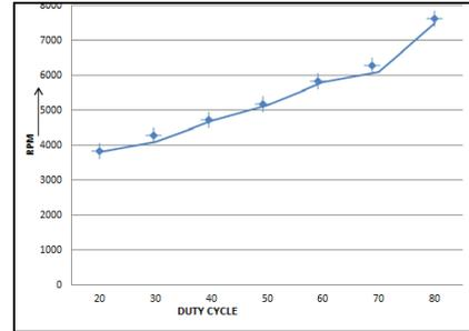
Fig. 7: Speed versus duty cycle curve
