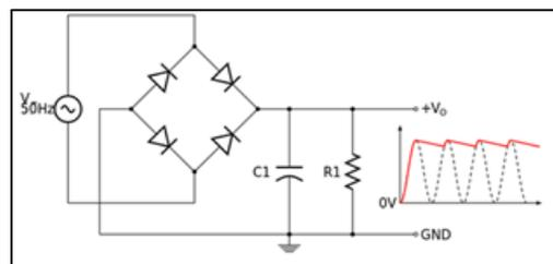
Fig. 2: Circuit diagram of bridge rectifier with Filter
