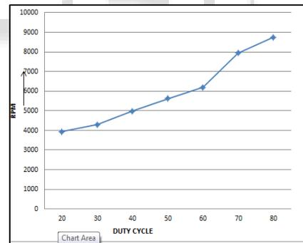
Fig. 8: Speed versus duty cycle curve
