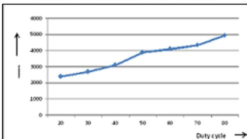
Fig. 6: speed versus duty cycle curve
