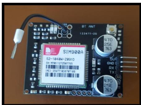
Fig. 5: SIM900A Dual band GSM/GPRS TTL Module
