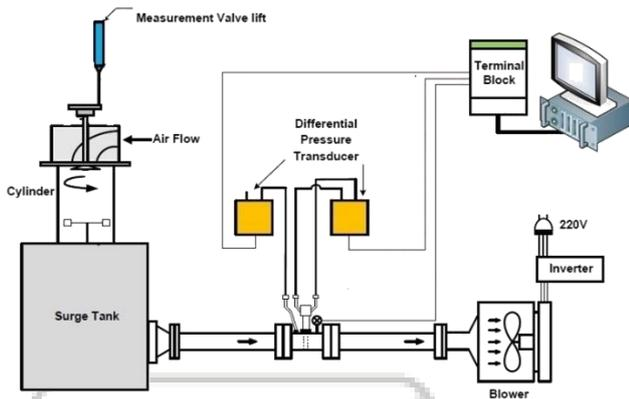
Fig. 2: Block diagram of setup
