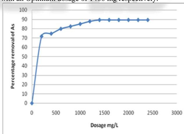
Fig. 5: Effect of Adsorbant dosage on Laterite soil
