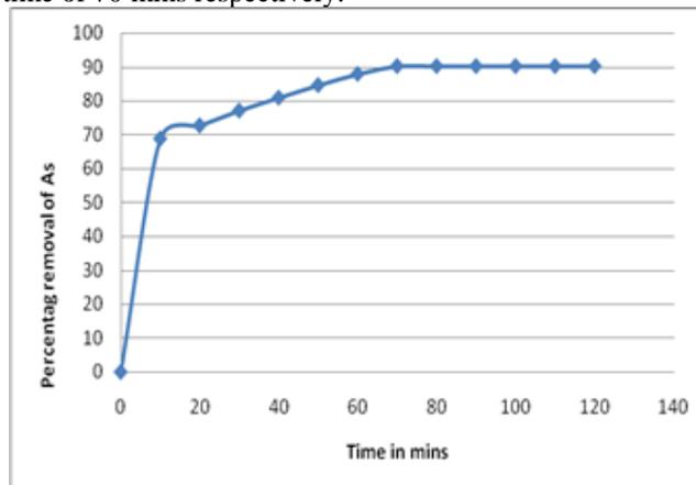
Fig. 4: Effect of Contact time on Laterite soil
