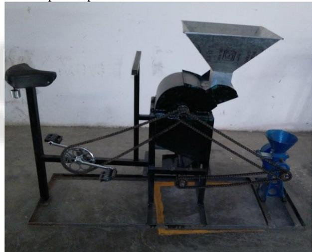
Fig. 2: Pedal operated Groundnut sheller and crusher Machine
