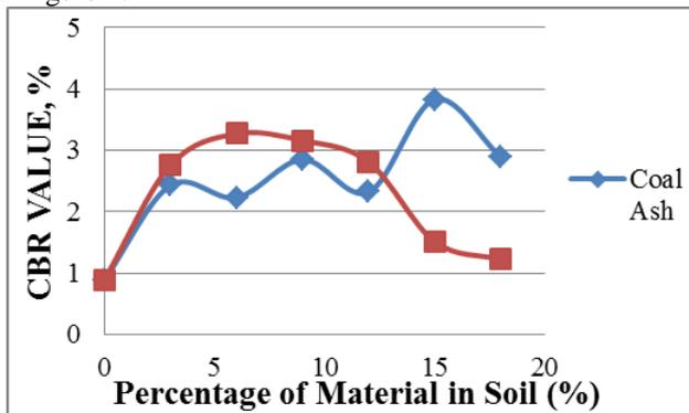
Fig. 4: Effect of Coal Ash and Stone Dust on CBR at Different Percentage
