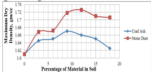
Fig. 1: Effect of Coal Ash and Stone Dust on MDD at Different Percentage
