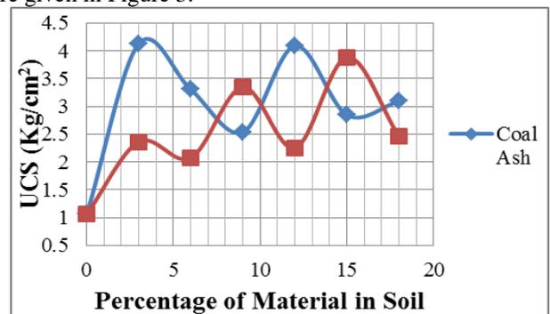
Fig. 3: Effect of Coal Ash and Stone Dust on UCS at Different Percentage
