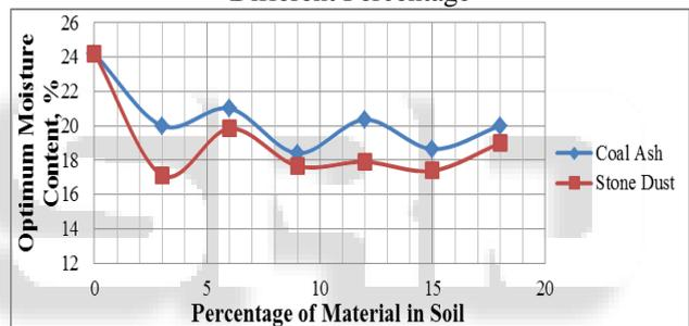
Fig. 2: Effect of Coal Ash and Stone Dust on OMC at Different Percentage
