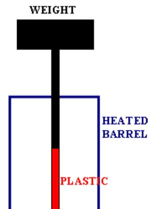
Fig. 3.6.3: Melt Flow Rate or Melt Flow Index
