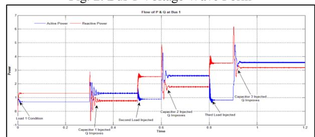
Fig. 3: Flow of active and reactive power at bus 1
