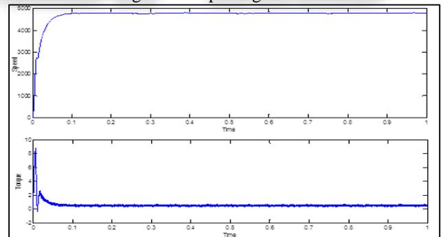
Fig. 5: Speed- Torque waveform (Without load torque)
