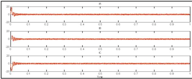
Fig. 7: stator current waveform (without load torque)
