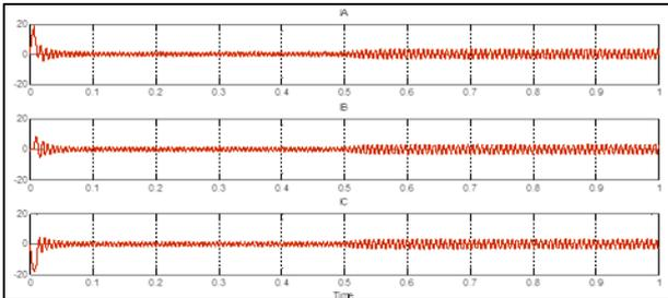
Fig. 8: stator current waveform (with load torque)
