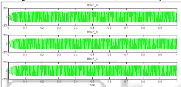
Fig. 9: Back emf waveform (without load torque)
