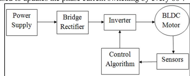
Fig. 1: Basic Block diagram of BLDC motor
