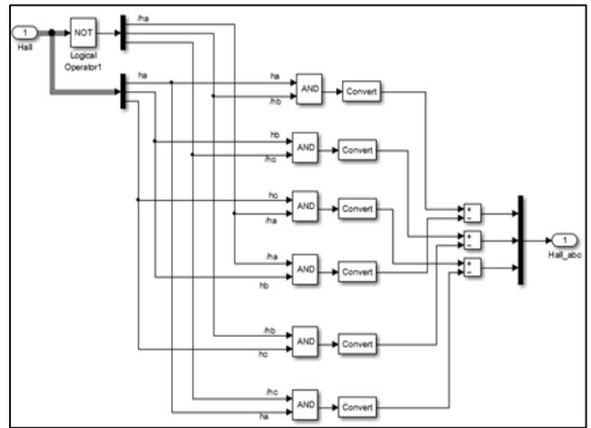
Fig. 3: Gate pulse logic operator
