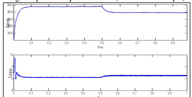
Fig. 6: Speed- Torque waveform (With load torque of 0.8N.m at  $t=0.5s$ )
