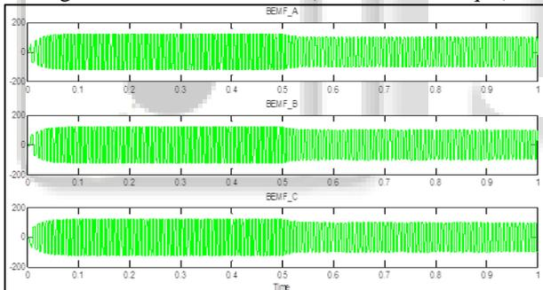
Fig. 10: Back emf waveform (with load torque)
