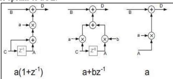
Fig. 2: Basic functional units of lifting schemes
