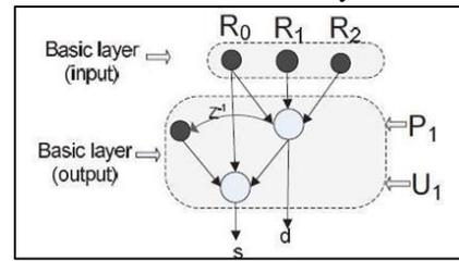
Fig. 3: Lifting structure for (5, 3) wavelet
