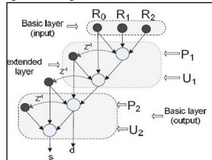
Fig. 4: Lifting structure for (9, 7) wavelet
