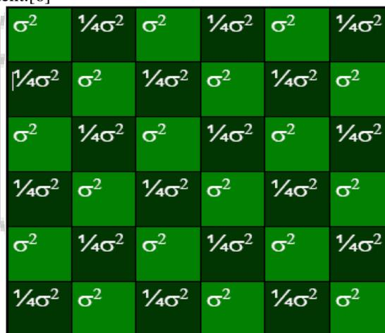
Fig. 1: When demosaicing is performed with linear interpolation, the original green pixels have higher variance than the interpolated green pixels. The spatial pattern of variances is the basis for detecting the presence of demosaicing. The green photosites pixel values in the Bayer array are IID with variance  $\sigma^2$ , the above image shows the variance from which each pixel value is drawn.
