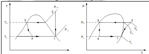
Fig. 9: T-S and P-H diagram
