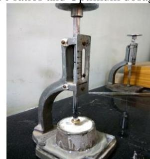
Fig. 2: Experimental setup for Penetration Test
