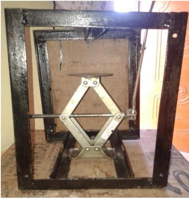
Fig. 2: Frame of machine with screw jack.
