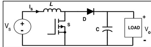
Fig. 3: Circuit diagram of Boost converter
