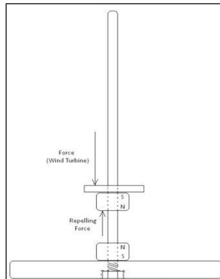
Fig. 5: Magnet Placement of Nd-Fe-B Magnet
