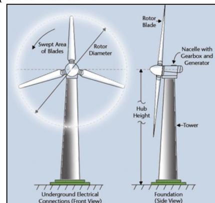
Fig. 1: Horizontal Axis Wind Turbines
