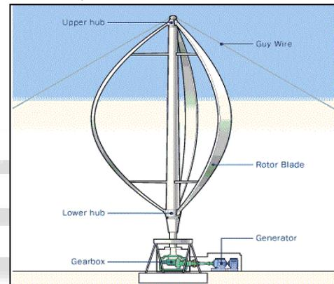
Fig. 3: Darrieus Vertical Axis Wind Turbine
