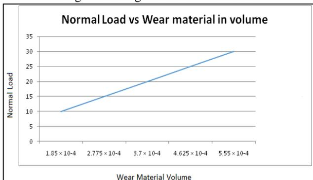
Fig 4: Normal load vs wear material in volume
