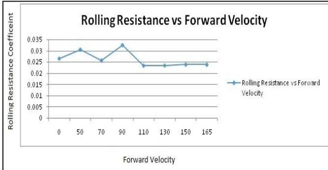
Fig. 2: Rolling resistance vs forward velocity
