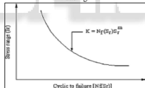
Fig. 2: A typical S-N Curve for constant amplitude test results.
