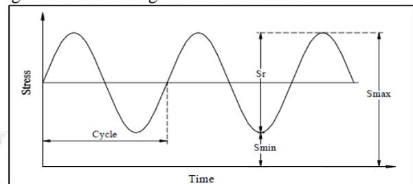
Fig. 1: A typical stress history for the constant amplitude loading.
