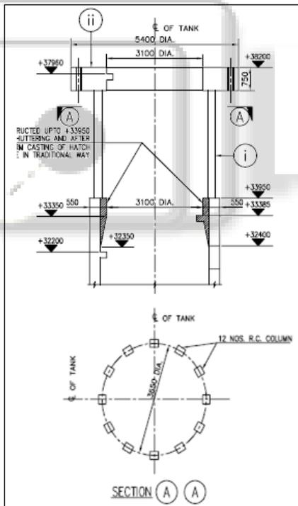
Fig. 2: Sectional Elevation Showing Stage-II
