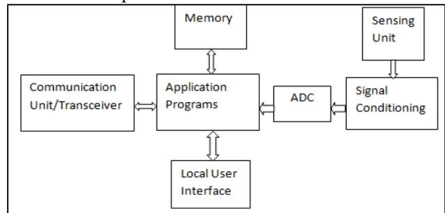
Fig. 2: Block Diagram of the E-way System
