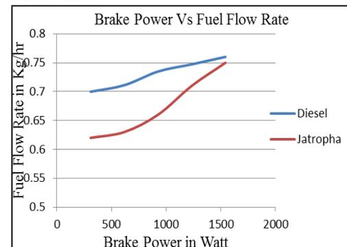
Fig. 3: Brake power Vs fuel flow rate for Diesel and Jatropa oil.
