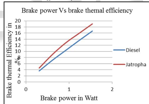
Fig. 2: Brake power Vs brake thermal efficiency for Diesel and Jatropa oil.
