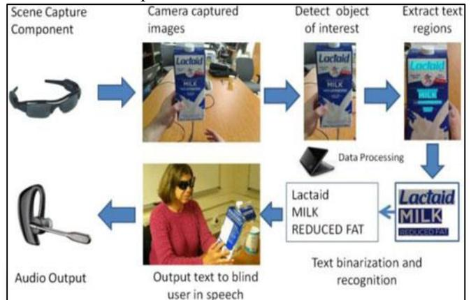
Fig. 3: Flowchart of the proposed framework to read text from hand-held objects for blind users<sup>[1]</sup>
