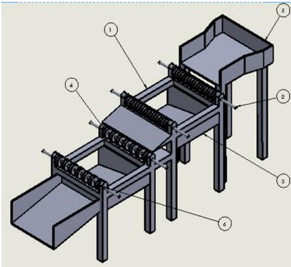
Fig. 3: Assembly of Tomato Sorting Machine
