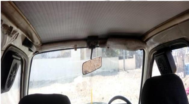
Fig. 3: Auto fan placed at opposite direction of each other In this condition after 1:30 PM one fan was stopped because in that direction solar PV sell not able to absorbed sun radiation. So in fig.4. shows temperature chart.
