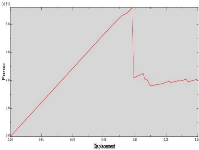
Fig. 4: Graph 6.1 Force (lb.) vs. Displacement (inch) for Plate with Hole
