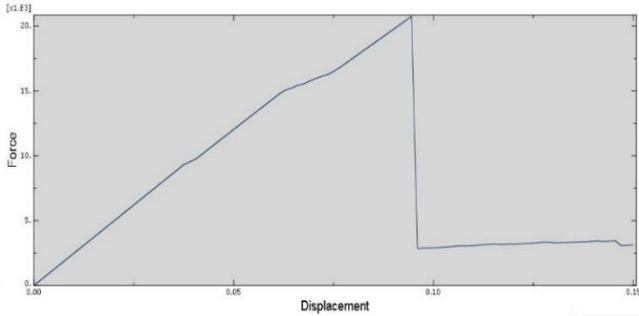
Fig. 10: Graph 6.6 Force (lb.) vs. Displacement (inch) for Plate without
