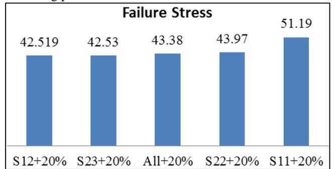
Fig. 7: Graph 6.4 Variation of Strength with Lamina Strength Parameters for Plate with Hole
