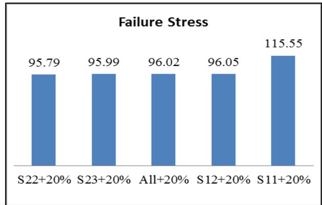
Fig. 13: Graph 6.9 Variation of the Strengths with the change in strength parameters for Plate without Hole
