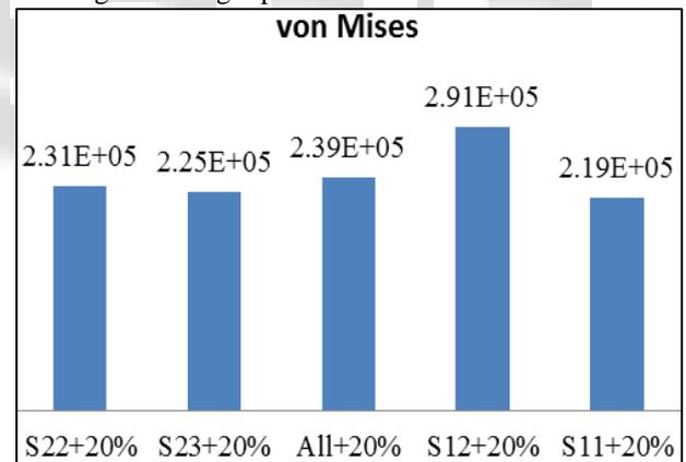
Fig. 14: Graph 6.10 Variation of the von Mises Stress with the change in strength parameters for Plate without Hole
