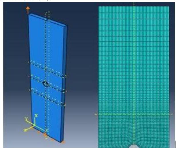
Fig. 2: Applied Boundary conditions and Meshing
