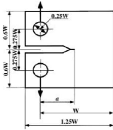
Fig. 8: Compact Tension (CT) Specimen
