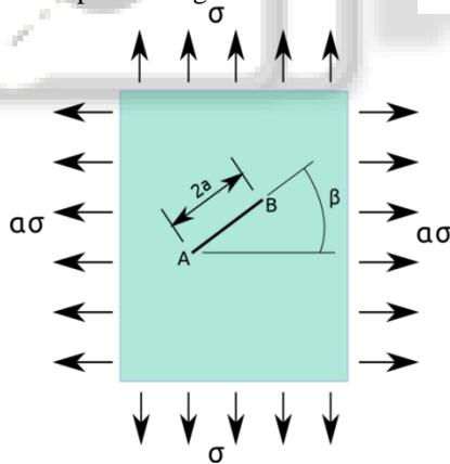
Fig. 3: Plate with Slanted Central Crack under Biaxial Load
