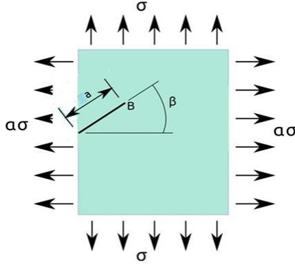
Fig. 2: Plate with Slanted Edge Crack under Biaxial Load
