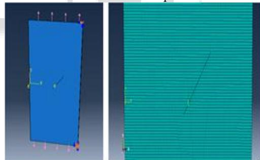
Fig. 7: Plate with Inclined Central Crack with Load, BC and Mesh in Abaqus
