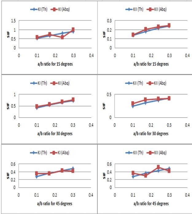
Fig. 13: Graph 4. SIFs for various angle cracks
