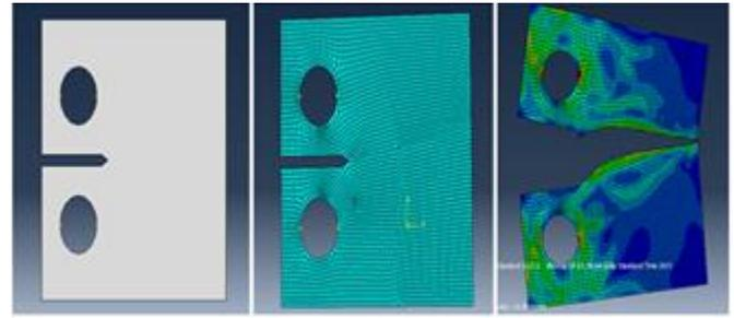
Fig. 10: Inclined Crack in CT Spicemen with Mesh and Crack Propagation path of in Abaqus
