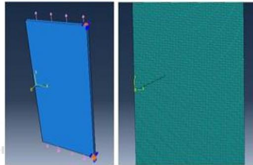
Fig. 6: Plate with Inclined Edge Crack with Load, BC and Mesh in Abaqus
