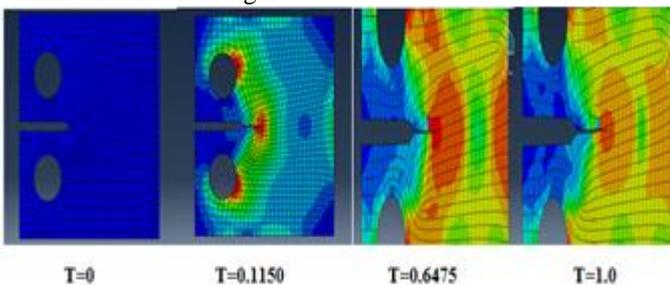
Fig. 9: Straight Propagating Crack in CT SPECIMEN with Mesh for various step Times in Abaqus
