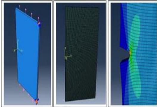
Fig. 4: Plate with Straight Edge Crack Along with Load, BC, Mesh and Analysis Results in Abaqus
