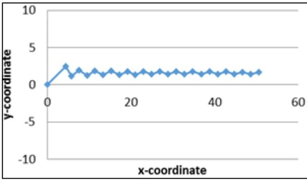
Fig. 18: Graph 8. Crack propagation path by Analytical Calculations using Matlab
