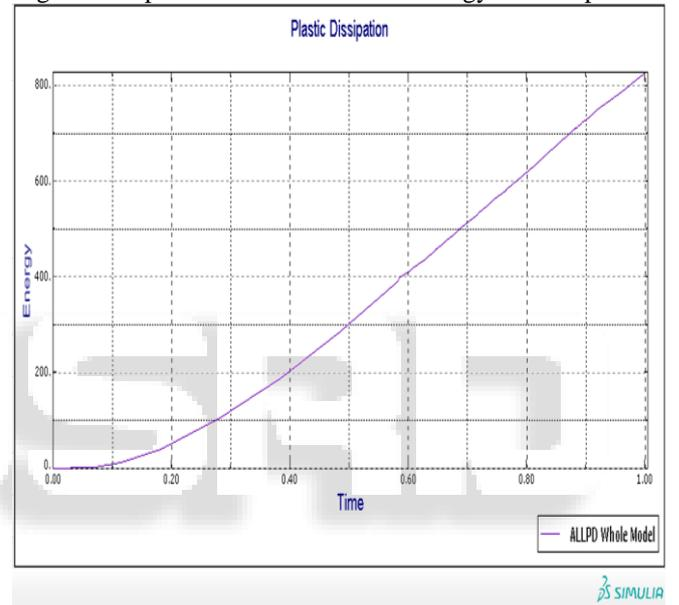
Fig. 16: Graph 7. Variation of Plastic Dissipation Energy with Step Time
