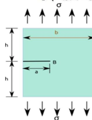
Fig. 1: Plate with Edge Crack Subjected to Uniaxial Load
