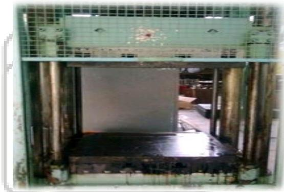
Fig. 2: Compression Molding Machine
