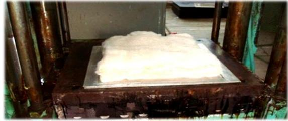
Fig. 3: Web placed on mould
