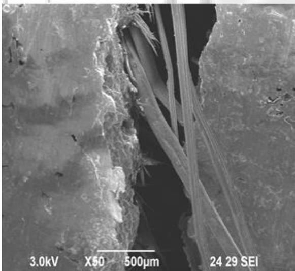
Fig. 6: SEM Image of Fracture surface of tensile strength of composite board
