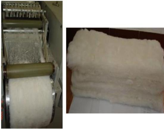
Fig. 1: Webs produced using the miniature carding machine
