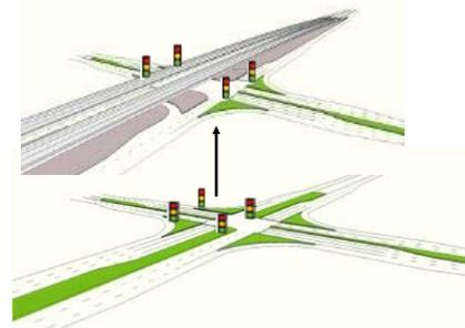
Fig. 1: Layout of an At-Grade Intersection Converted To a Flyover-Improved Intersection
