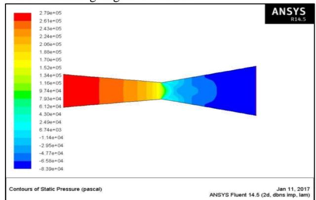
Fig. 5: Contours of Static pressure
