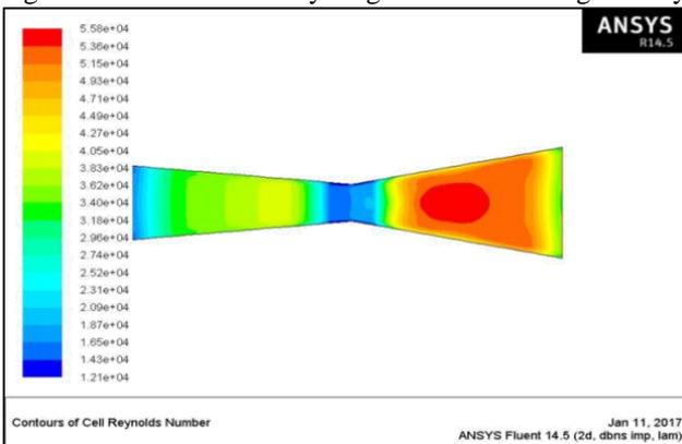
Fig. 9: Contours of Cell Reynolds number of nozzle geometry.
