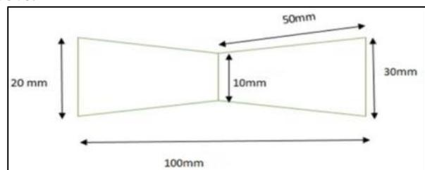
Fig. 2: Geometry of the nozzle
