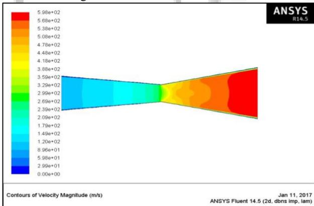
Fig. 8: Contours of velocity magnitude of nozzle geometry.
