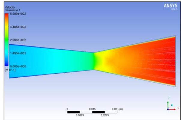
Fig. 10: Velocity stream line of nozzle geometry.
