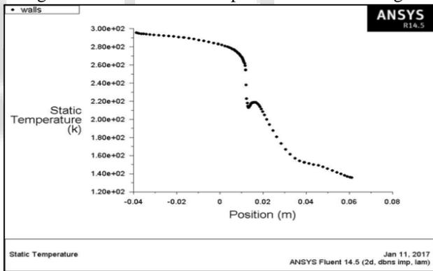
Fig. 12: Plot between static temperatures to nozzle length
