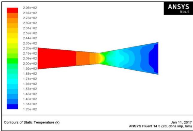
Fig. 6: Contours of static temperature
