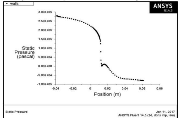
Fig. 11: Plot between static pressure to nozzle length
