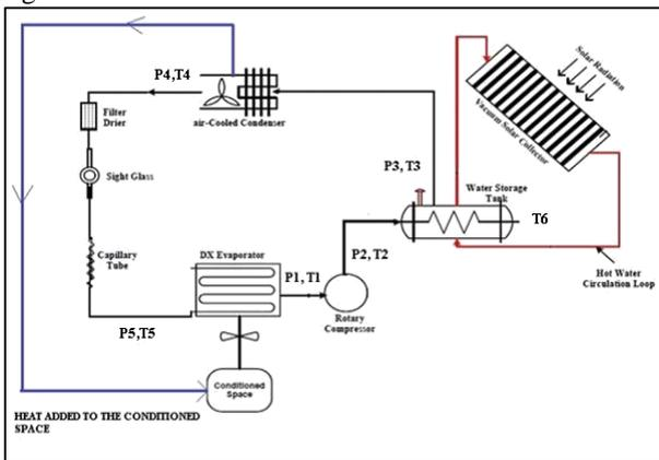
Fig. 1: Line diagram of Experimental Setup
