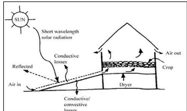
Fig. 4: Indirect Solar Dryer.
