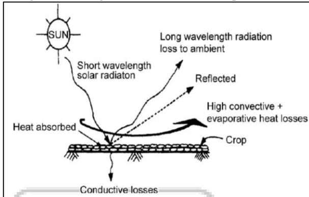
Fig. 2: Open Solar Dryer
