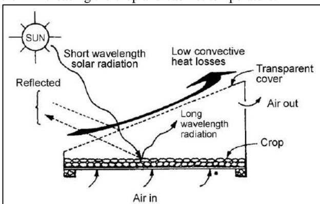
Fig. 3: Direct Solar Dryer
