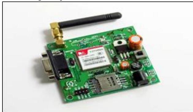
Fig. 7: GSM SIM900A
