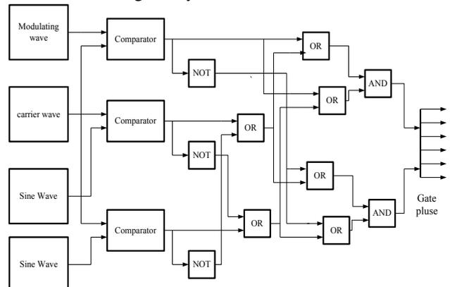
Fig. 5: Control circuit of MBC method in Matlab/Simulink
