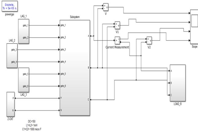
Fig. 6: Power Circuit of Three phase Inverter
