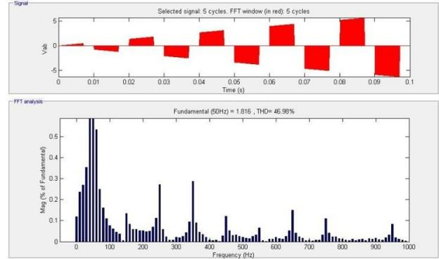
Fig. 9: THD of Line to Line Voltage Vab
