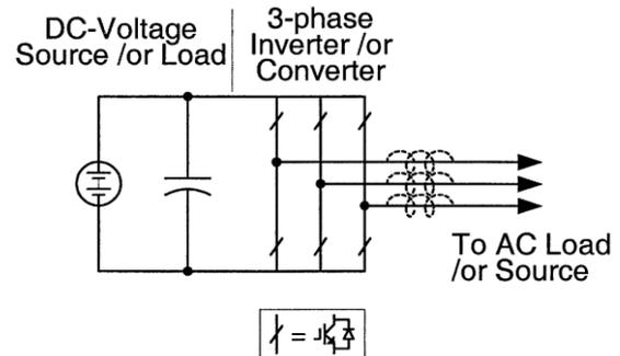
Fig. 1: Traditional Voltage source converter
