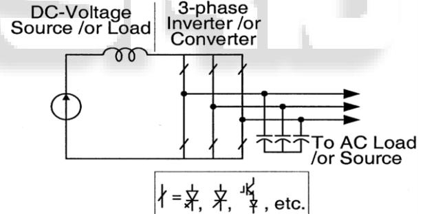
Fig. 2: Traditional Current source converter
