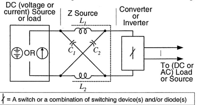
Fig. 3: General structure of Z-Source inverter
