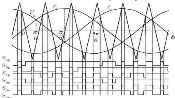
Fig. 4: Maximum boost control method
