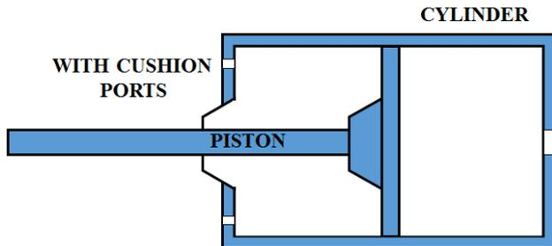
Fig. 2: With Cushioning Mechanism
