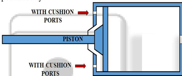
Fig. 3: with Cushioning end position
