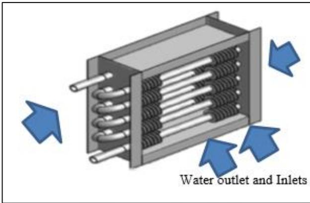
Fig. 1: Serrated spiral fin and tube heat exchanger
