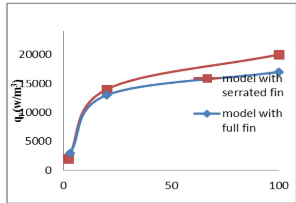
Fig. 3: Performance plot of cases with and without fin serration
