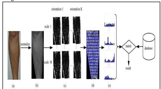
Fig. 2: Schematic diagram of proposed algorithm.(a) Original Image (b) Normalized Image (c) Gabor Magnitude (d) Orientation Field (e) Histograms
